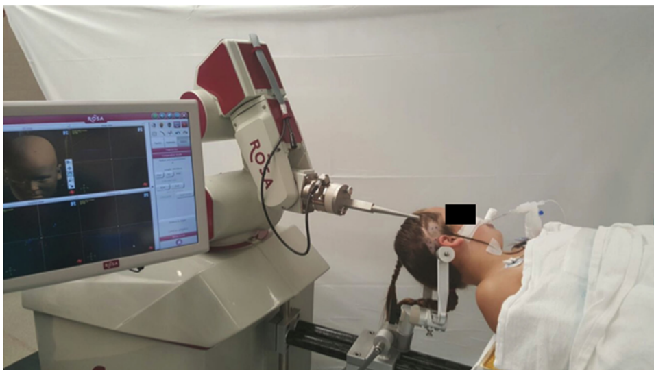
FIG. 1. Operating room configuration of the ROSA system. The patient's head is secured in a Mayfield head holder that is attached at a fixed position to the ROSA robot. The robotic arm can freely move around the patient's head to the entry point of planned stereo-EEG trajectories. In this case, all planned trajectories are in the right temporal region.
